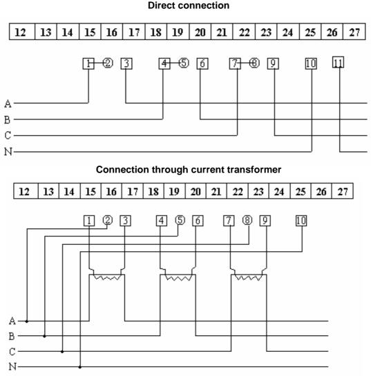
Connection through current transformer and voltage transformer
